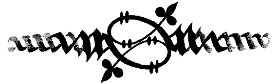
Fig. 3. Spring lancet following spring release.
